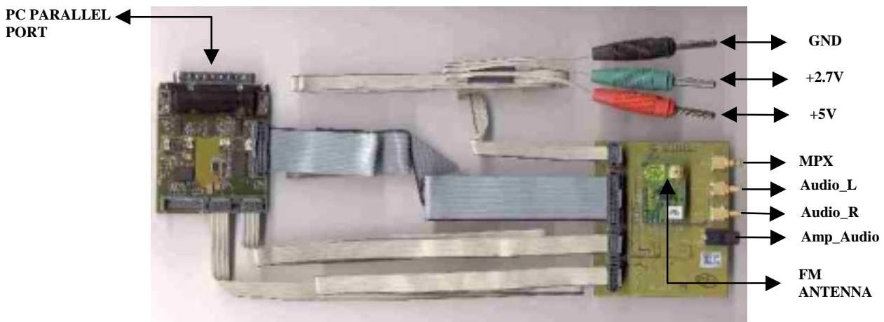
Figure 34 connection of TEA5767/68 demo board
